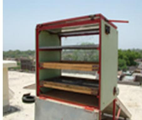
Trans Solar Technologies introduces a new cabinet type multipurpose solar dryer, which can be used for vegetable/fruit drying, grain drying, cooking, cloth drying etc. Results for making powders of moringa leaves, tomato and potato powders, green chilly powders etc. are excellent.
