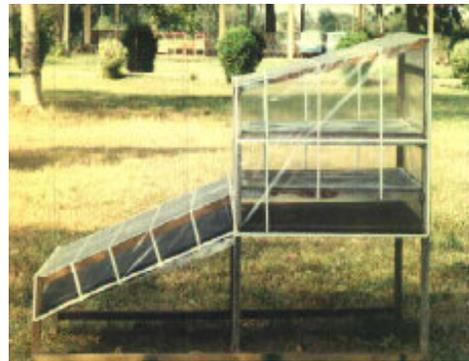
Completed Solar Cabinet Dryer – 2 m<sup>2</sup> model
